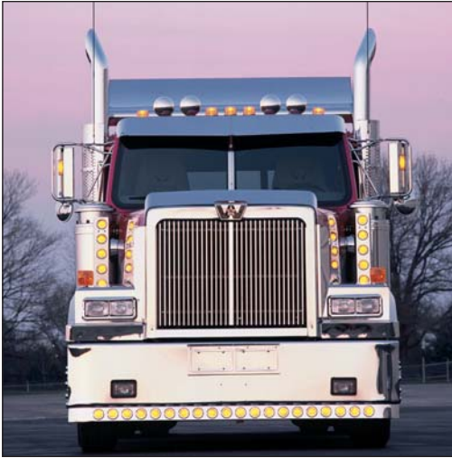
The LowMax cab has been lowered nearly a foot from standard configurations, for an overall height under 104" with lights and horns removed and 275/70 R22.5 tires.
